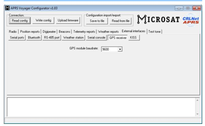
• "GPS module baudrate" - selection of GPS receiver communication baudrate.
