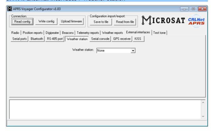
• "Weather station" - selection of weather station model connected to APRS Voyager serial port.
