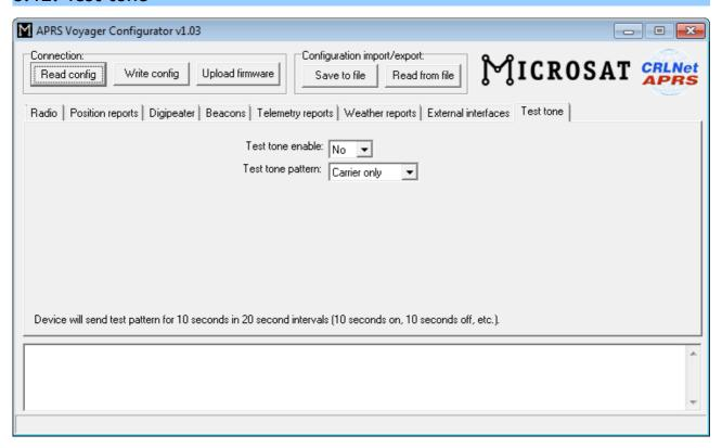
This Tab allows to enable test tone generation in APRS Voyager. When test tone is enabled, device will not send and receive any packets. Alternatively it will send a constant test pattern with 50% duty cycle in 20 seconds interval (10 seconds on, 10 seconds off).
