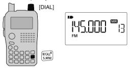
② Push and hold **[S.MW]**(M/CALL) for 1 sec. to enter select memory write mode.
