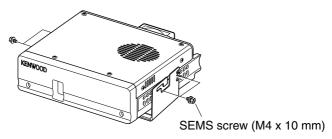
• Set an appropriate angle for the TX/ RX unit, using the 3 screw slots on the rear edge of each bracket side.
