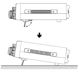
*Note*: Do not use the wire stand as a carrying handle, as it could slip out of its mount, causing the transceiver to be dropped! Use the carrying handle on the side of the FT-847 for transport purposes.
