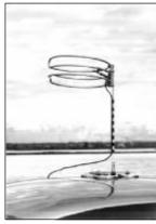
Photo Horizontal Loop for SSB/CW Operation
