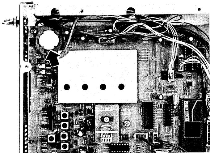
Fig. 9 Lithium Battery Location
