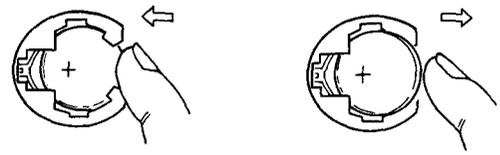
Slide cell inward, then pry up to eject
