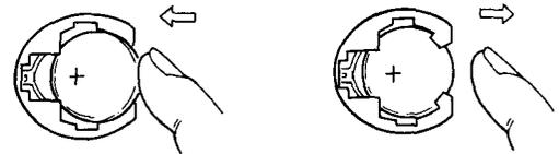
Slide cell downward through slot, then inward to release
