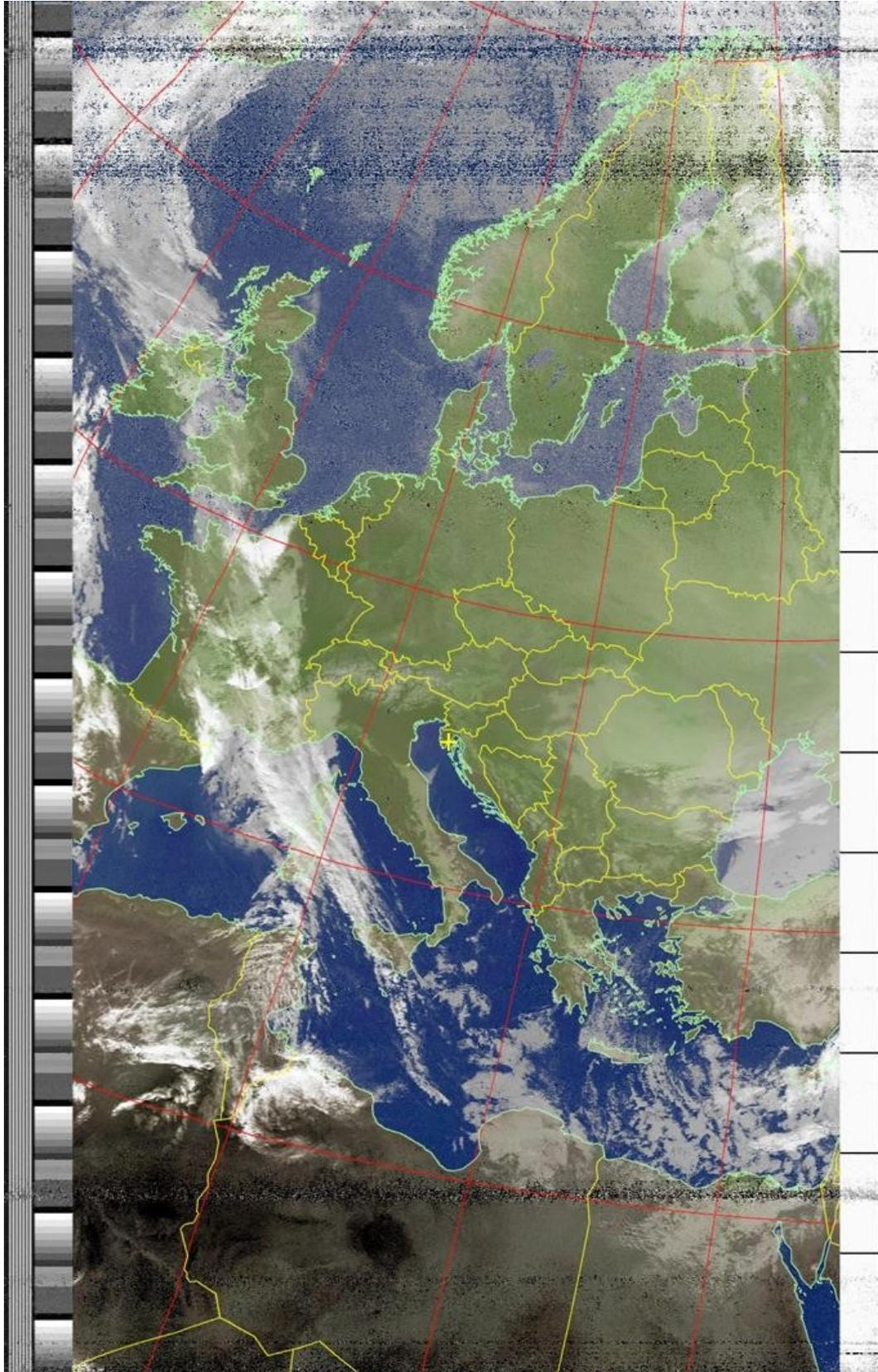
Second test was made using the advanced setup. V-dipole antenna and an FM-notch filter with the LNA4ALL with a Bias-T and ESD protection modification on the antenna. The same coaxial length and the RTL.SDR v.2 dongle.
