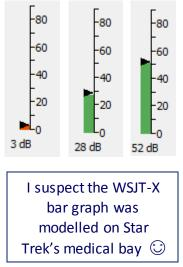
The bar graph bar should normally be green. showing acceptable levels. If it is red, the level is probably too high (causing distortion, apparently wide signals and poor copy) or too low (no input, no signals to copy!).
