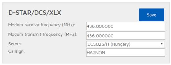
You can use this connector to connect openSPOT to a network which supports the DCS protocol.
