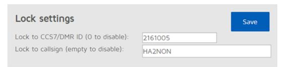
This block is only available in advanced mode. It allows you to lock openSPOT to the given CCS7/DMR ID and/or callsign. If lock is enabled, openSPOT's modem will only allow calls originating from the given ID or callsign.
