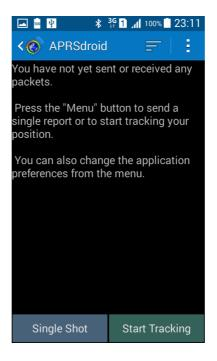
Press on "Start Tracking" and you should get a confirmation that connection was opened correctly. Your PLXTracker red/green led should start to blink in green. After some time you should start to see received packets:
