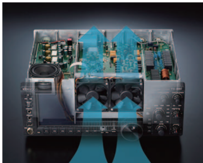
Fig. 85 Fan Placement and Ventilation Flow
