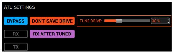
**BYPASS** - Tuner's bypass mode.
