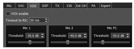
VOX system triggers when the microphones voice signal exceeds the **Threshold**. The **Threshold** could be set for each microphone individually.
