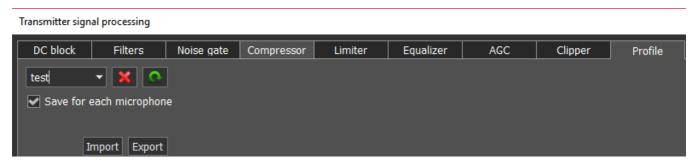
In the **Profile** tab, you can save settings of the whole TX processing module in a separate module, independent from the main software profile. Load PROC settings from a file by pressing the **Import** button and save a profile in a file by pressing the **Export** button.
