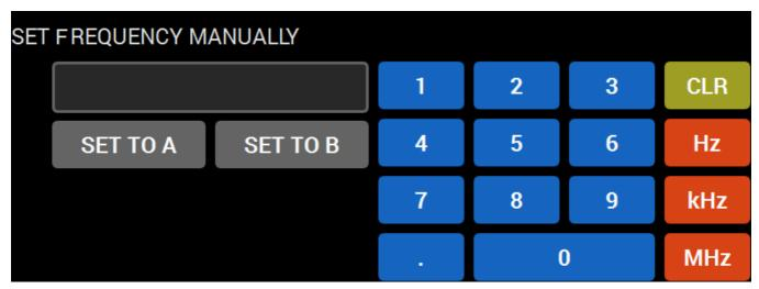
Enter the required frequency either with touchscreen or with physical buttons on the front panel, then apply the entered frequency either to VFO A (SET TO A) or to VFO B (SET TO B).
