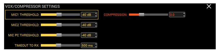
MIC1 THRESHOLD, MIC2 THRESHOLD, MIC PC THRESHOLD - VOX system trigger thresholds.
