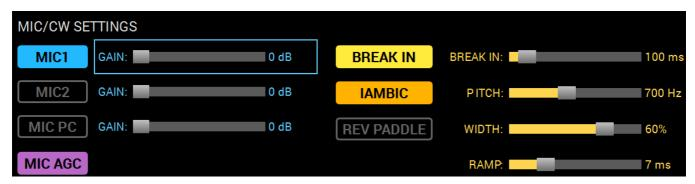
Press the MIC button on the the front panel of the transceiver to select the required microphone input MIC1, MIC2, MIC PC.
