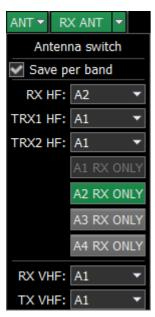
**Antenna switch** menu. This menu allows you to lock the required HF/VHF antenna input **only for RX**. When the certain HF/VHF antenna input is locked for RX you cannot select it for TX.
